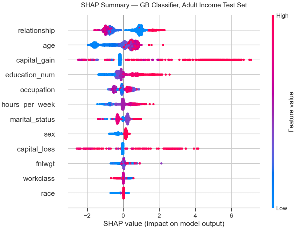
Figure 17.7: SHAP summary plot for the Gradient Boosting classifier on the Adult Income test set (log-odds scale). relationship is the strongest predictor, with high feature values (e.g. “Husband”) pushing log-odds of > \$50K upward and low values (e.g. “Own-child”) pushing strongly negative. age has the second-widest spread, contributing positively at high values and negatively at low. capital_gain shows the longest positive tail: a small fraction of observations with very high capital gains receive extreme SHAP values extending past 6. capital_loss similarly produces a wide spread in both directions. education_num contributes near-monotonically — higher education consistently increases the predicted probability of high income. fnlwgt , workclass , and race contribute relatively little.
